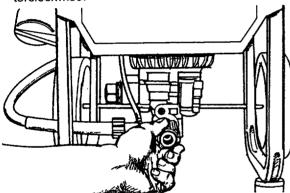
Slide the nozzle forward when you wish to adjust the spray to low pressure mode. Slide the nozzle backward to achieve high pressure (see "Adjusting the Spray Pattern in figure below).
